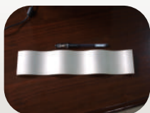
工件材料:SKD11 Workpiece Materials 工件厚度:70 Workpiece thickness 粗糙度 Ra:0.9um Roughness
