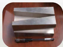
工件材料:SKD11 Workpiece Materials 工件厚度:140/40°切割 Workpiece thickness:140/40° Taper 粗糙度 Ra:1.2um Roughness
