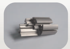
工件材料:SKD11 Workpiece Materials 工件厚度:30 Workpiece thickness 粗糙度 Ra:0.95um Roughness
